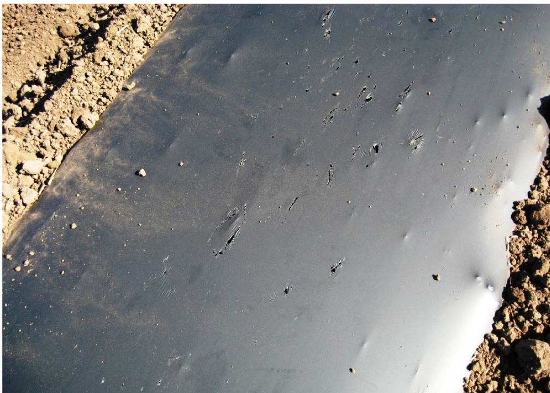
Figure 26, left: An example of the damage caused to both 12 and 15 micron thicknesses of Mater-Bi® during laying operations (S. Heisswolf).
