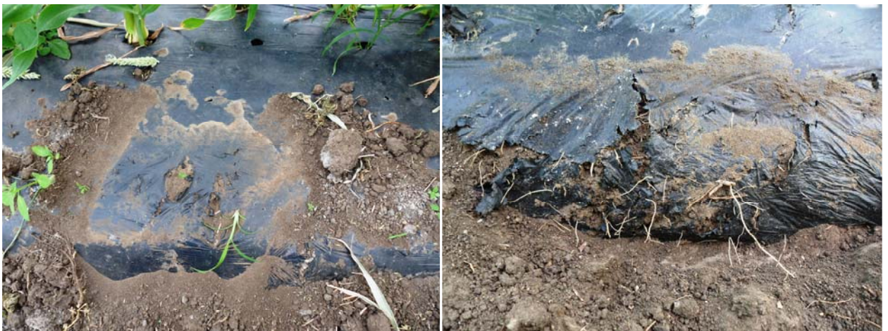
Figure 47, left: Biodegradation of above ground surfaces of 15 micron Mater-Bi® where soil and leaves were resting on the surface, promoting microbial activity, and Figure 48, right: Below ground degradation of 15 micron Mater-Bi® showing evidence of microbial activity, 14 weeks after laying (S. Limpus).
