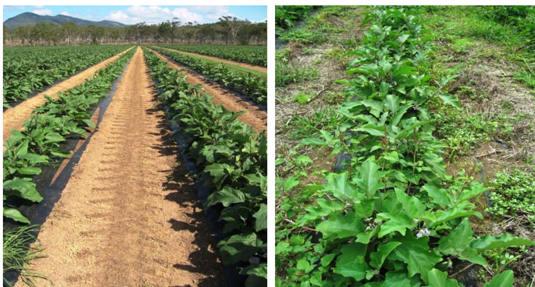
Figure 41, left: Splitting observed in 15 micron Mater-Bi ® mulch film planted with eggplants, 12 weeks after laying, and Figure 42, right: The left side of bed is still largely intact after 25 weeks, with the right or northern, sun exposed side has lost significant bed coverage (S. Heisswolf).
