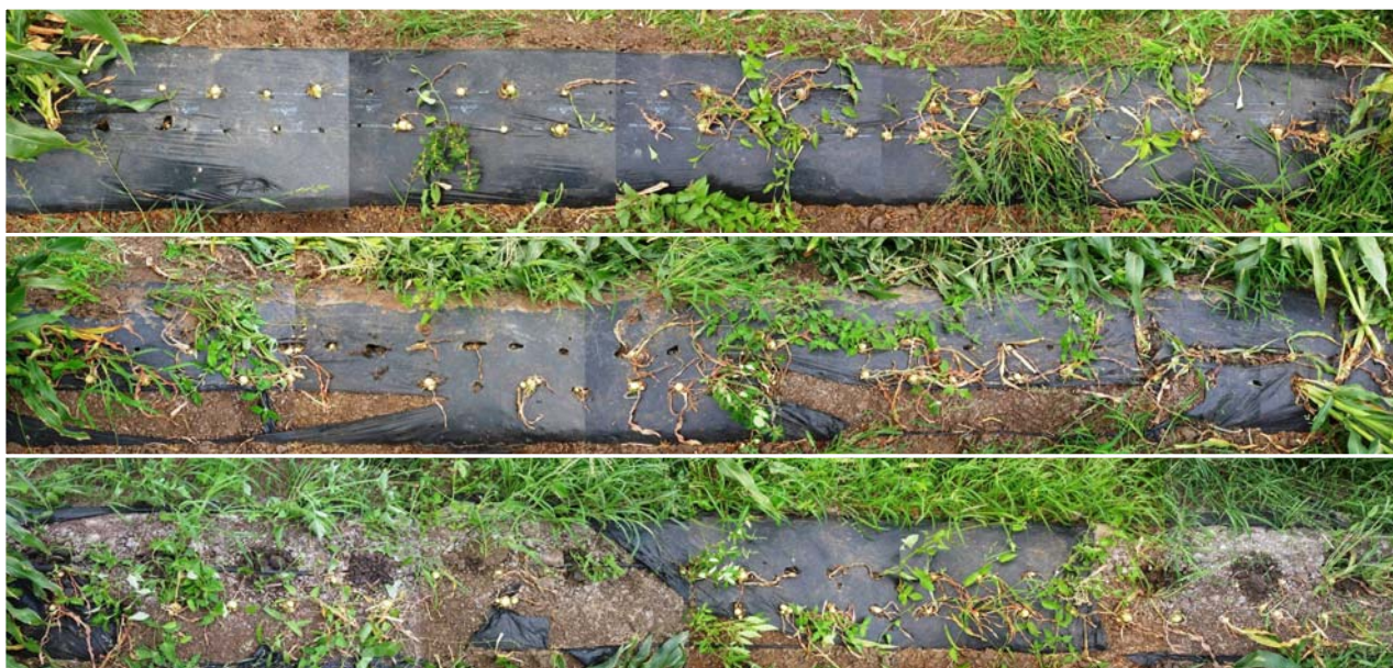
Figure 49, top: Polyethylene film bed in sweet corn retaining 99% bed cover at harvest some 16 weeks after initial laying, Figure 50, middle: 12 micron Mater-Bi® bed coverage declined to 80% at harvest, and Figure 51, bottom: 12 micron Mater-Bi® bed coverage declined to 35% by harvest (S. Limpus).
